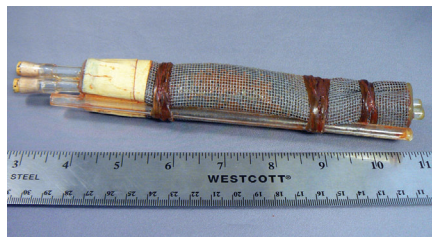
One of the first spiral wound RO membrane prototypes created at General Atomics in 1965
